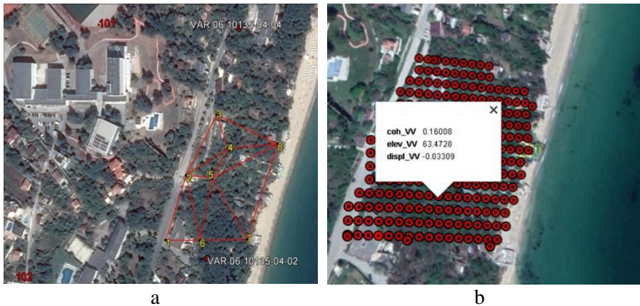
Figure 3: Picture of landslides region and GNSS network (a) and sampling network for SAR data (b).
