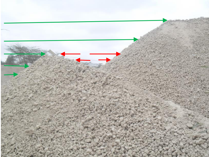
Figure 1: Laser scanned positions shown with arrows in green, positions that have been missed out ("shadowed") shown by arrows in red; the observer is at the left hand side of the heap in the figure.
