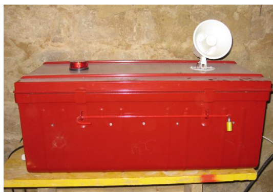
Illustration 8: Box for central computer and control system inclusive alarm system (optical and acoustical)
